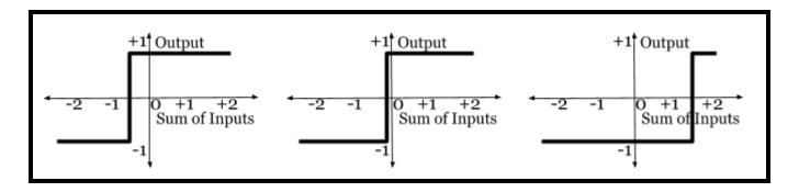
3. To describe the shape of a **step function**, we must specify three parameters: the **minimum** and **maximum** outputs, and the **transition** value where the output changes. (The figure above shows 3 step functions with different transition values.) Explain which of these parameters could be replaced or modified with an extra input value.
