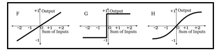
1. An **activation** (or **transfer**) **function** converts the weighted sum of input values into an output value. Use the 3 functions shown above to answer the questions below:
